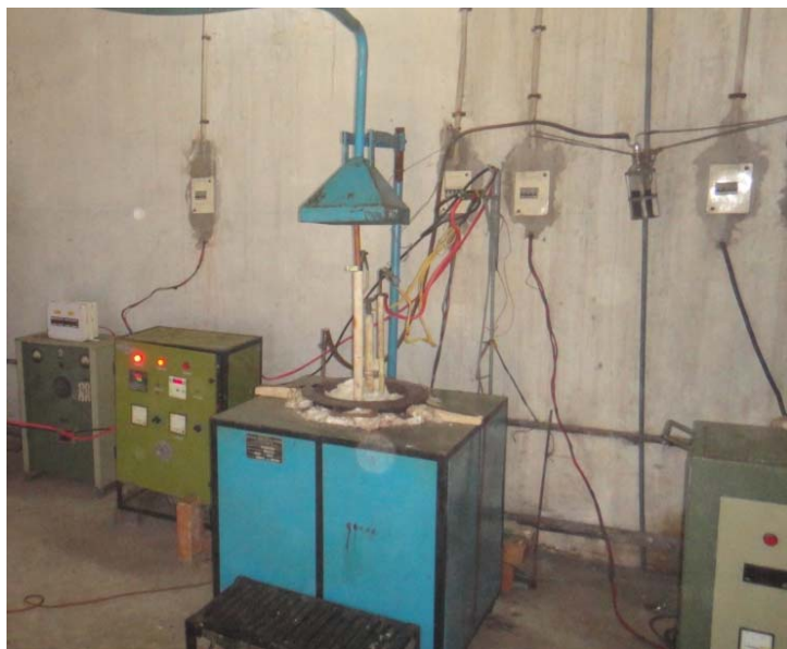
Electrolyser 100A Capacity
