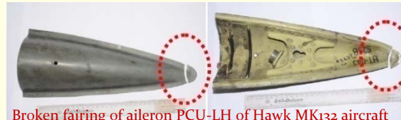
Broken fairing of aileron PCU-LH of Hawk MK132 aircraft
